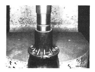
5 Coat mounting bore of sliding ring seal in bearing housing sliding ring with sealing compound.
