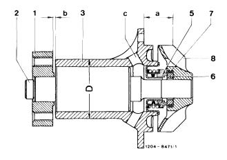
The water pump of engine 617.912 has a bearing diameter of 40 mm. In the event of repairs, install the water pump used up to now.
