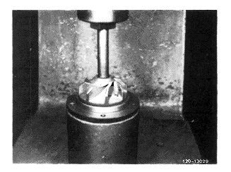
3 Remove counter-ring from impeller.
