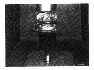
10 Heat fan hub on a hot plate to approx.  $300^{\circ}$ C (annealing color dark — up to light blue).
