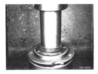
6 Coat O-ring on counter-ring with brake cylinder paste and push with chamfered side (arrow) into thorougly cleaned impeller.
